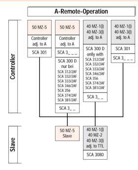
In the Metz A remote mode the master flashgun (controller) mounted on the camera controls the slaves in such a manner that automatic operation covers all slave units. The exposure is controlled by the sensor i on the controller. To implement this mode, all 40 MZ-.. slave units must first be fitted with an SCA 3080 Slave Adapter (available as an optional extra). 50 MZ-5 slaves do not require a slave adapter.
